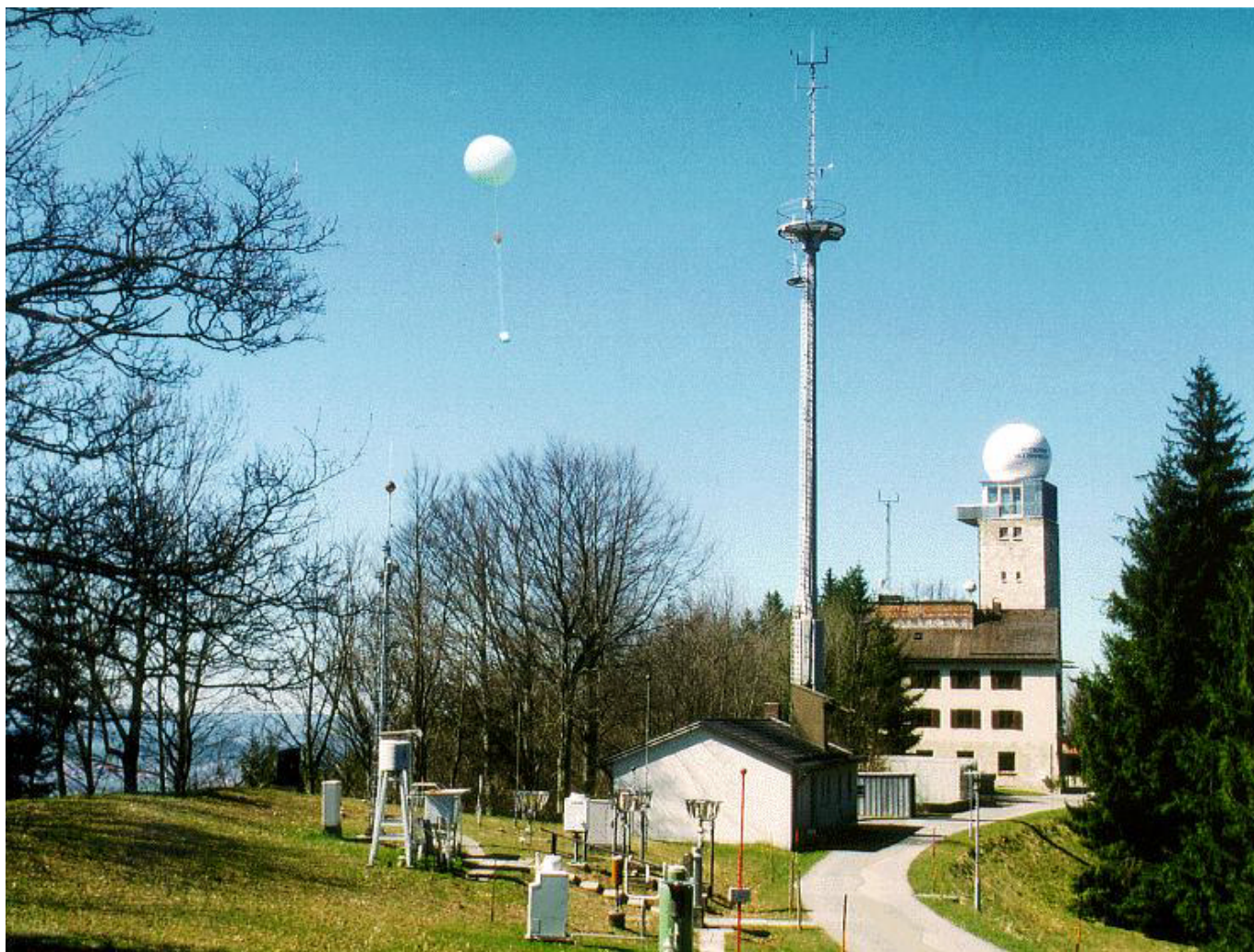
Figure 3. An ozonesonde being launched from the Hohenpeißenberg observatory, Germany.
