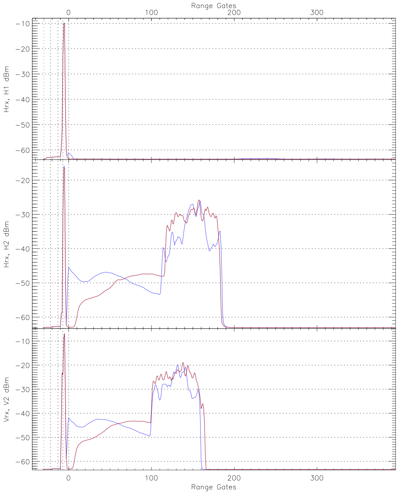
WCR2 CPP Averaged Received power for all recorded gates blue: 142405-143337, 10584 profiles averaged red: 143337-144308, 10584 profiles averaged
