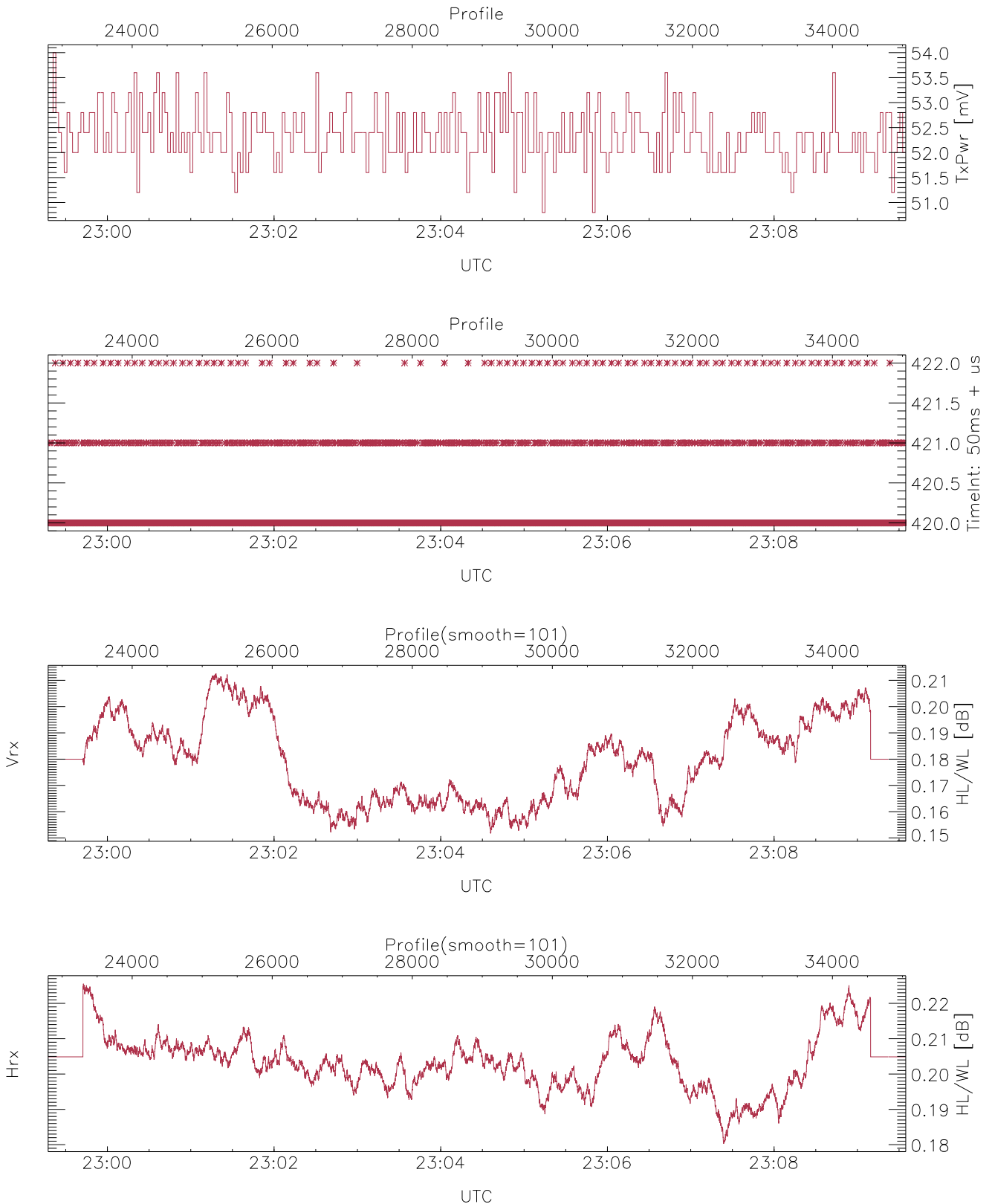
WCR2 CPP Tx Power Monitor, Profile Time Interval, HotLoad/WarmLoad Ratios
