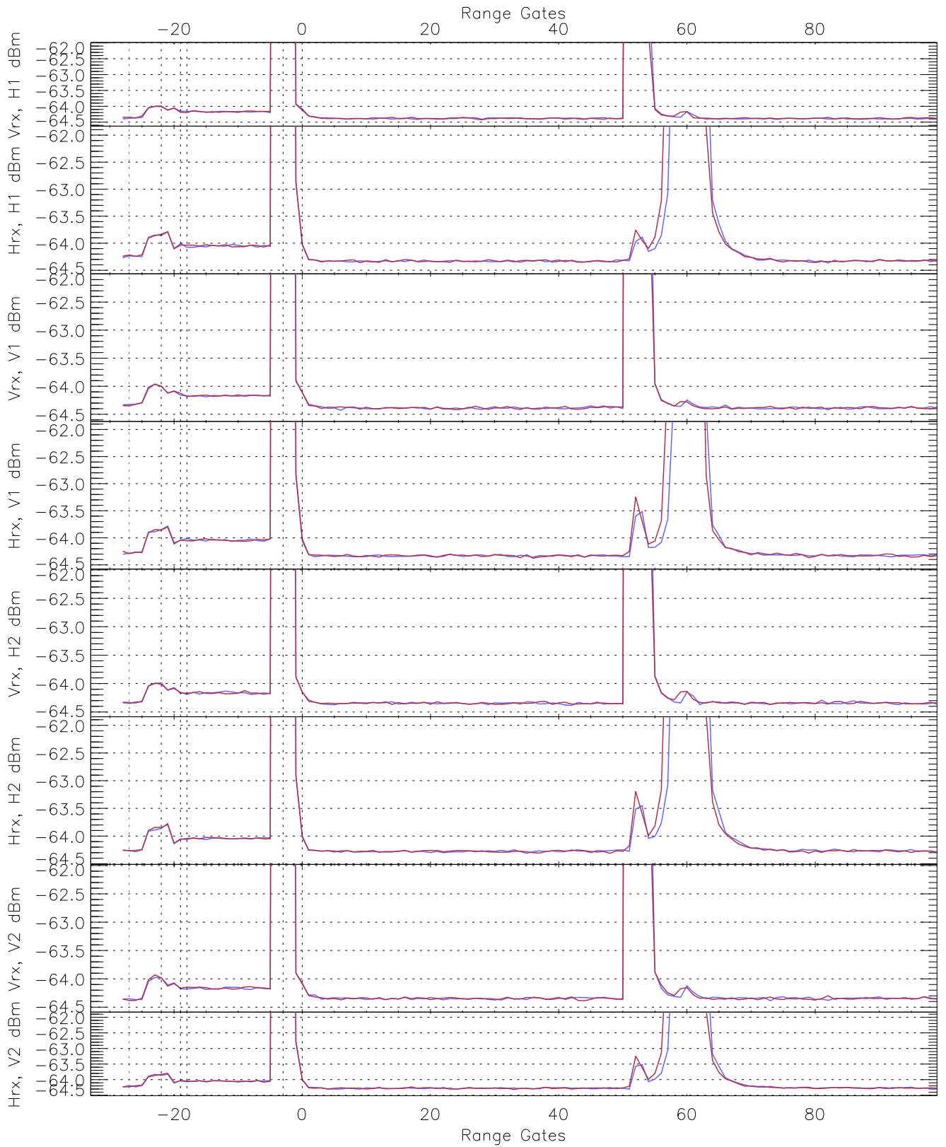
WCR3 FF4 Averaged Received power for the negative gates and up to 100 gate blue: 173407-173443, 102 profiles averaged red: 173443-173519, 101 profiles averaged
