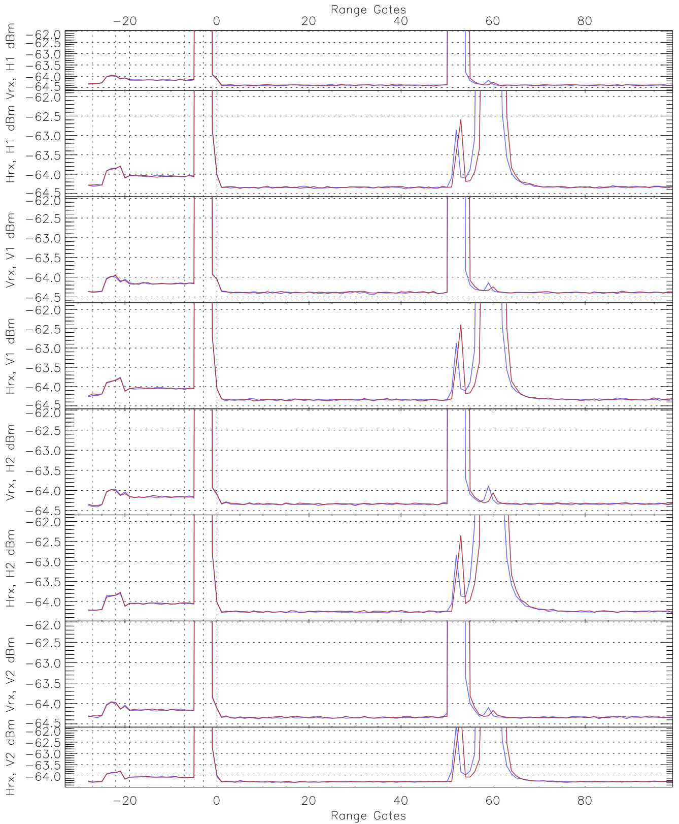
WCR3 FF4 Averaged Received power for the negative gates and up to 100 gate blue: 173916-173956, 155 profiles averaged red: 173956-174035, 155 profiles averaged
