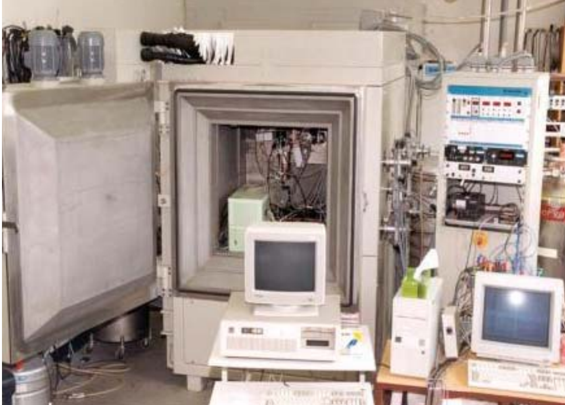
Figure 3: Environmental Simulation Facility for Ozone Soundings
