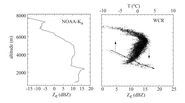
Fig. 15. Average reflectivity from vertical profiles measured by the NOAA Ka-band radar (left panel) and reflectivities measured by the WCR during the spiral ascent and descent (right panel) on Sept. 6, 1995.
